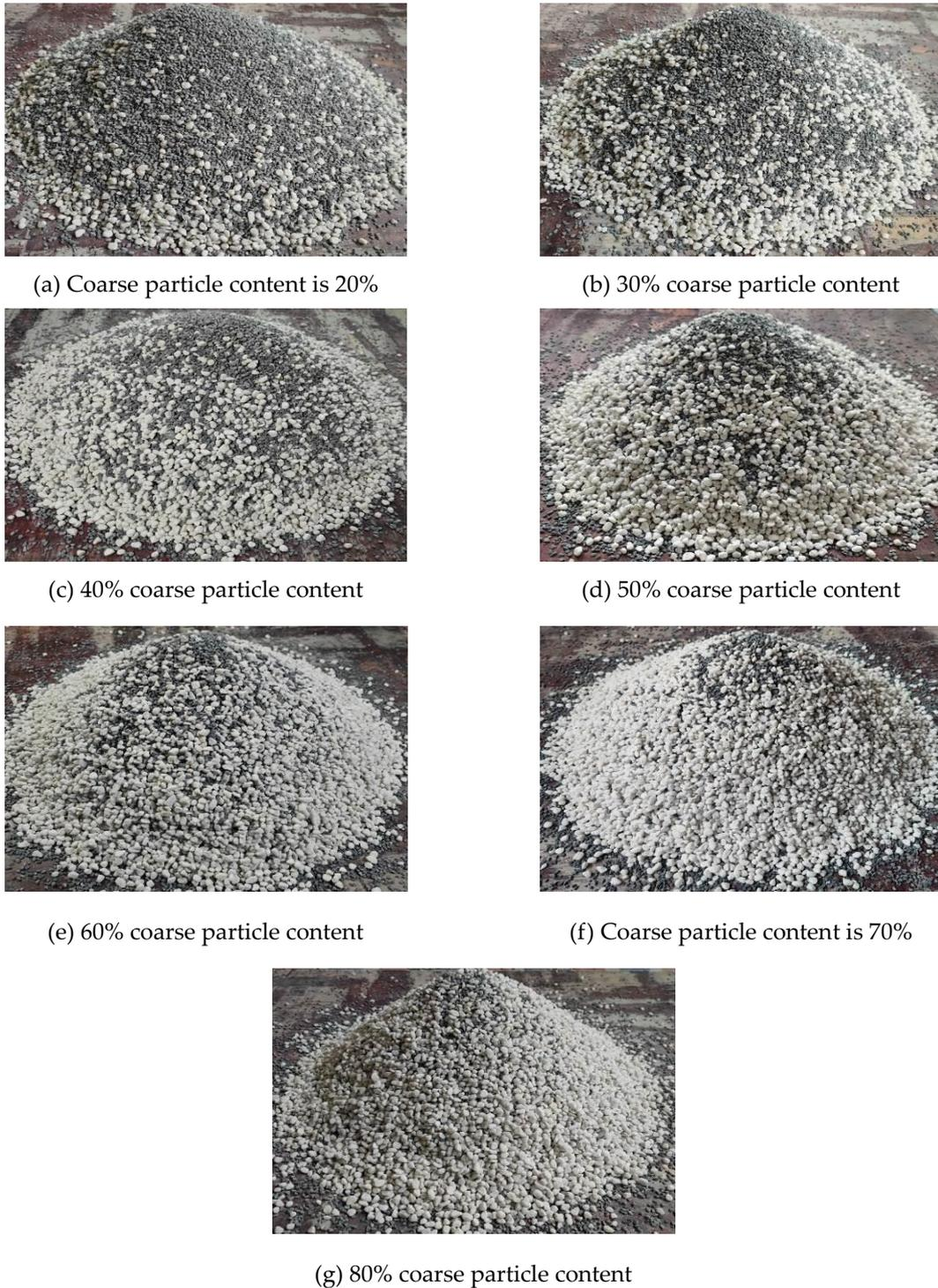
**Figure 3.** Oblique view of 3d stacking of binary irregular particle mixtures
