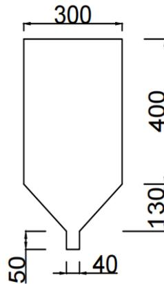
(a) Indoor test device diagram
