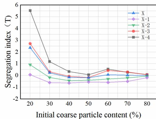
**Figure 11.** The particle segregation curve on the surface of granular heap
