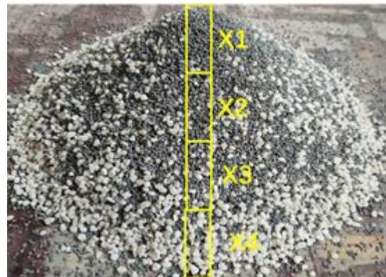
**Figure 7.** Schematic diagram of sampling position on the surface of the accumulation
