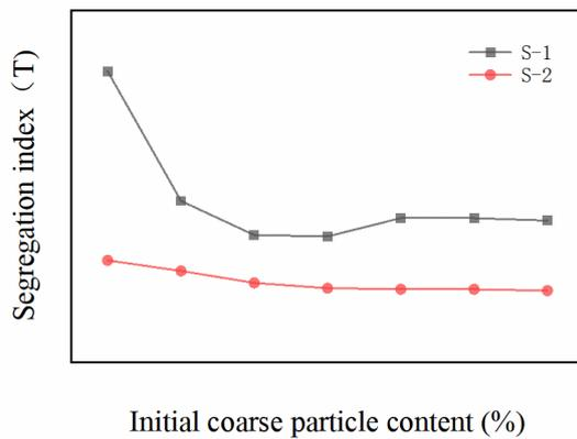
**Figure 10.** Segregation curves of particle heap from top view
