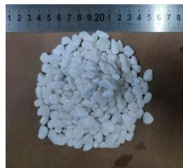
(c) White crushed stone 6mm-9mm
