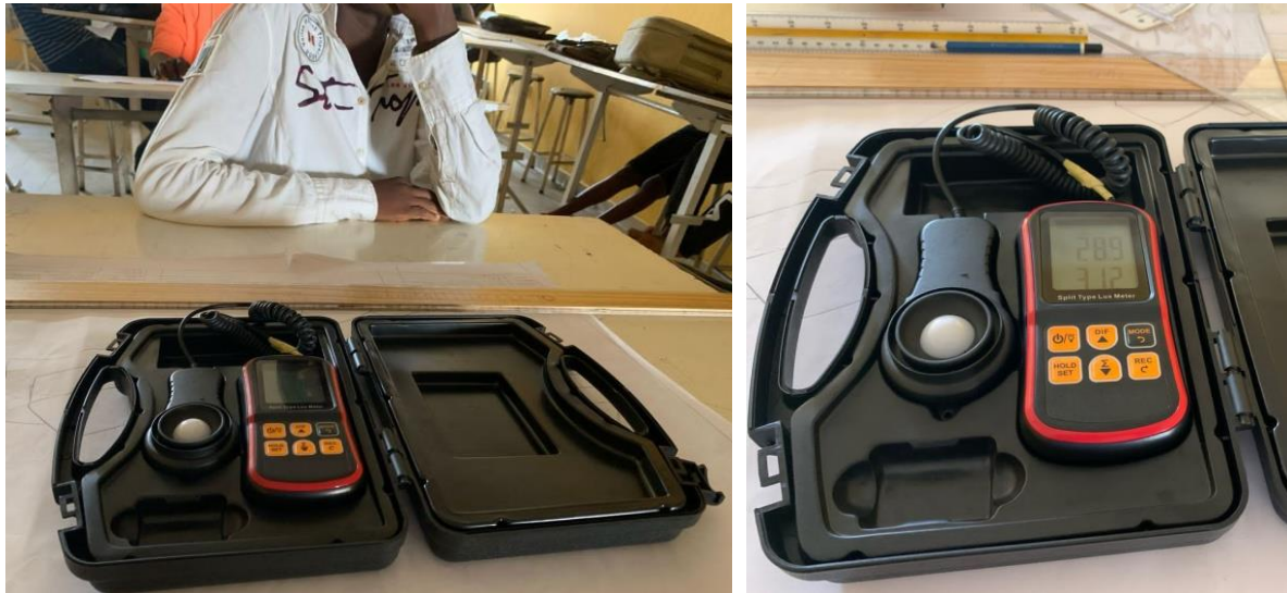
Plate 2. Picture showing the split type lux meter used to take readings in the studios
