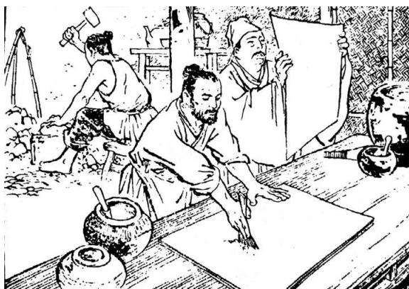
Figure 2. Illustration of powder-coating technique, from History of Papermaking (造紙史話), 1983.
